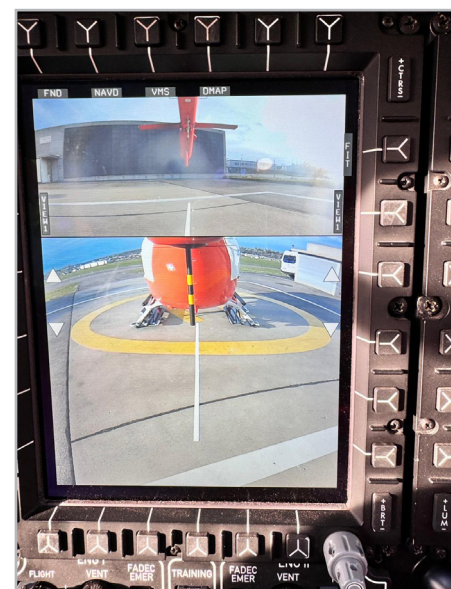
Fig. 3a / 3b: Signs on the tarmac indicate the correct magnetic heading (here: 030) to improve situational awareness
