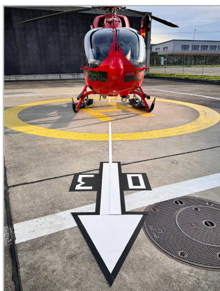
Fig. 3a / 3b: Signs on the tarmac indicate the correct magnetic heading (here: 030) to improve situational awareness
